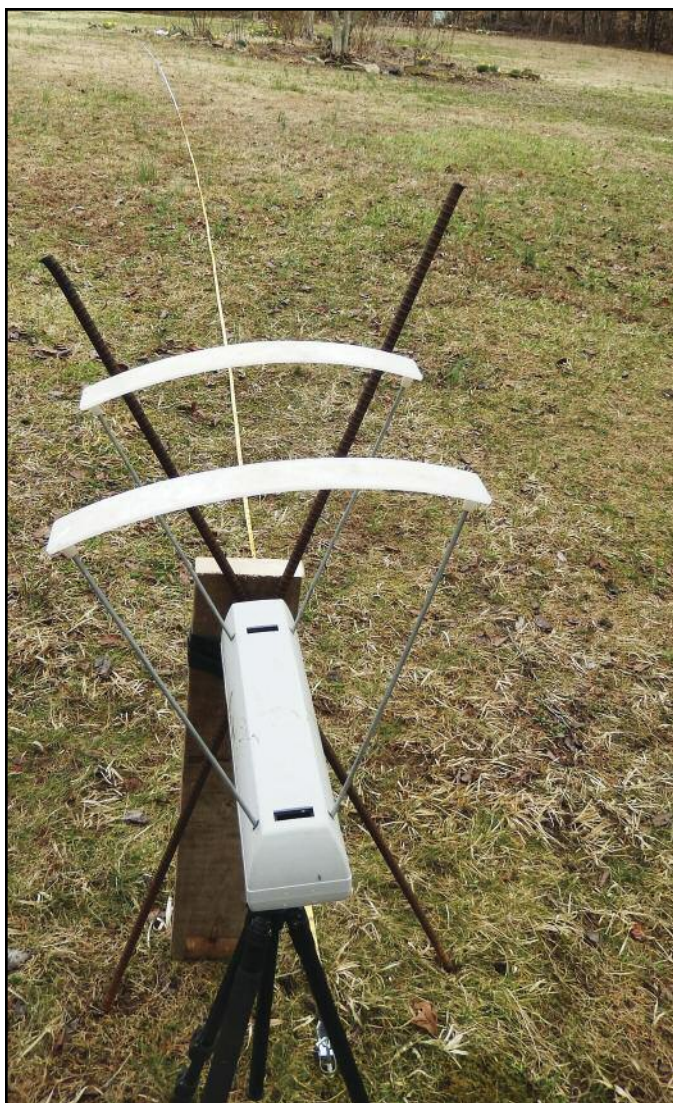
The author's chronograph set up for testing the speed under controlled conditions of both helical and straight fletching.
